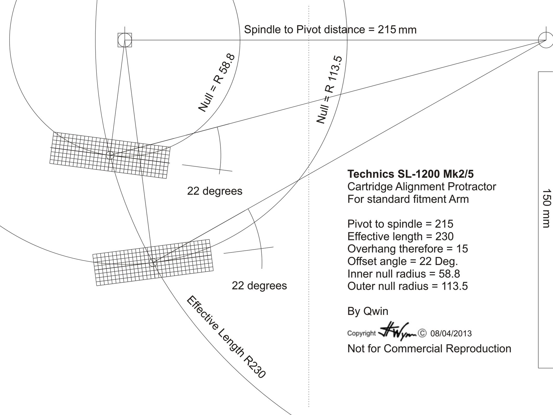
Spindle to Pivot distance = 215 mm
