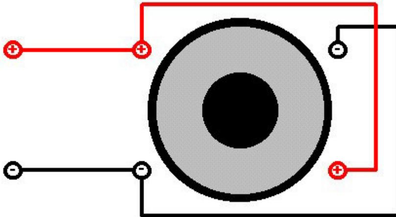
This method of wiring is the most common for DVC wiring. For our dual 8-ohm voice coil drivers, it results in a nominal 4-ohm load (parallel connecting voice coils of the same impedance results in half the impedance of either voice coil). This maximizes the output of our home plate amps, and also produces an impedance compatible with most car stereo equipment.
