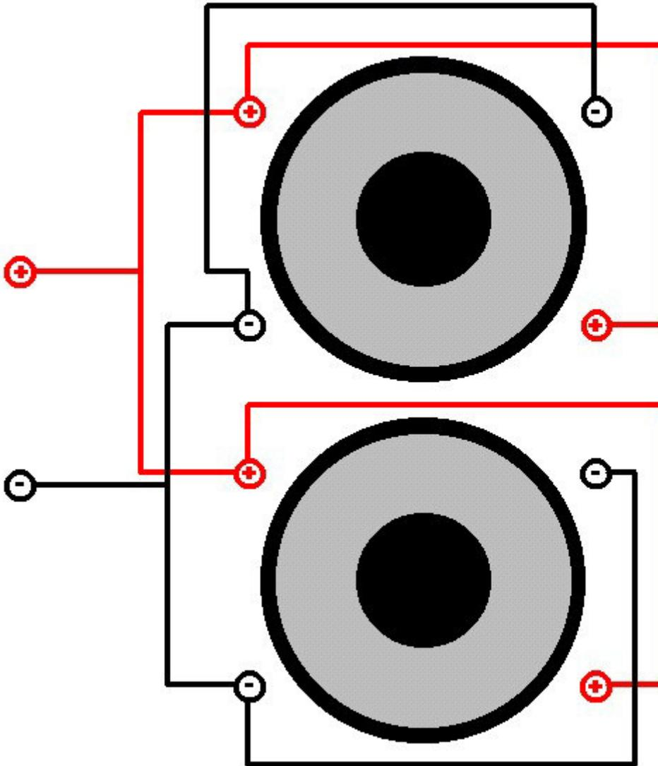
Note that all the positive terminals are connected together, and all the negative terminals are connected together. The total load, assuming dual 8-ohm voice coil drivers, is 2 ohms.
