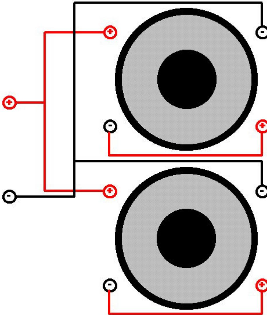
This results in a final 8-ohm load, assuming each driver has dual 8-ohm voice coils. While this may not "maximize" power output of an amp optimized for a 4-ohm load, it will result in more linear output for the same power input as a single driver.
