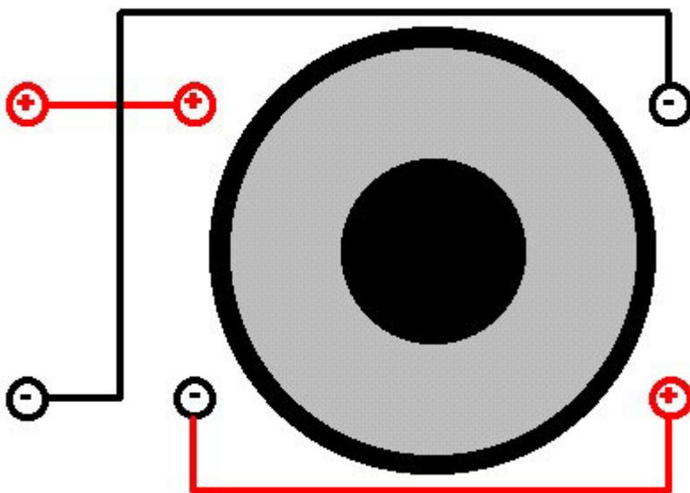
This method of wiring is not as widely used as the parallel case. For our dual 8-ohm voice coil drivers, it results in a nominal 16-ohm load (series connecting voice coils results in the sum of the impedances of all voice coils). This means of wiring is often used when wiring DVC drivers for use in large arrays, or in prosound applications (where 16 ohm loads are widely used).
