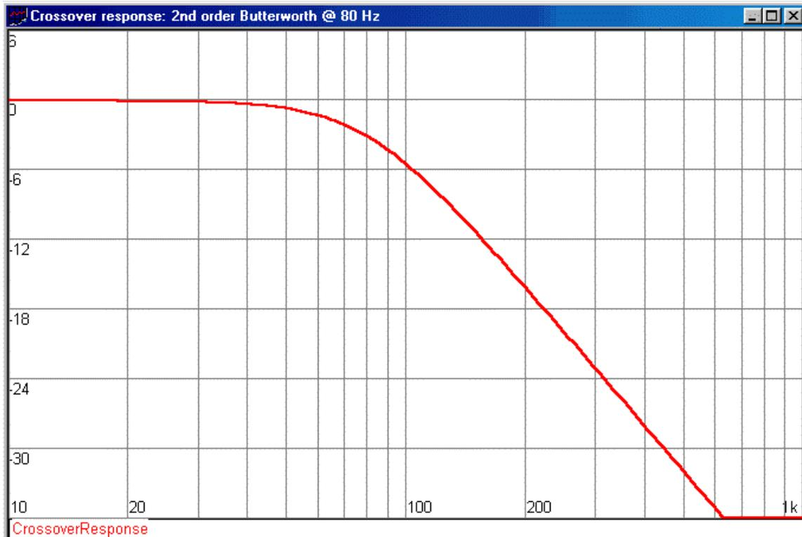
As you can see, the response of the crossover is never above 0 dB; in fact, above 20 Hz, the crossover is actually reducing the output of the nominal system. It is because of this effect that one needs to consider the crossover when designing a subwoofer system.
