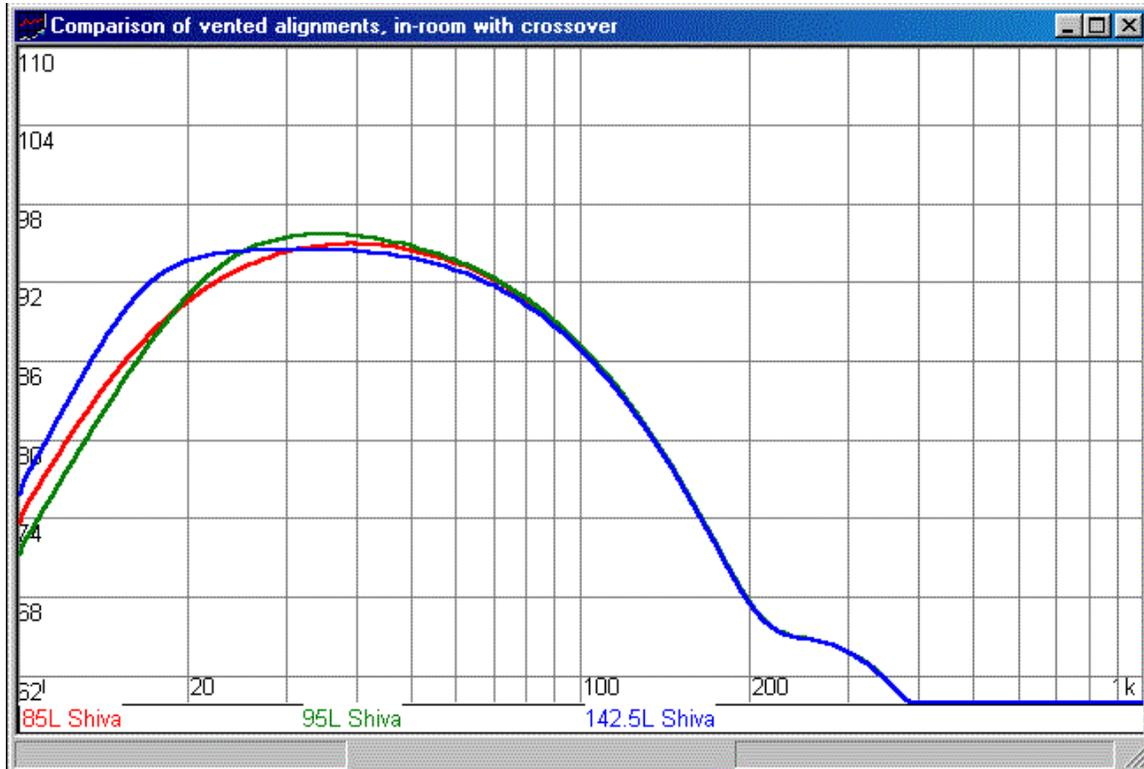
As can be seen, the EBS alignment is clearly the bass extension champion. Response is essentially flat from crossover to 16 Hz, with little peaking or “bowing” in the response. Additionally, the EBS has a major advantage in terms of SPL output down in the sub-20 Hz range. If the size of the box can be tolerated, or organ music is the reproduction goal, this is the recommended alignment.
