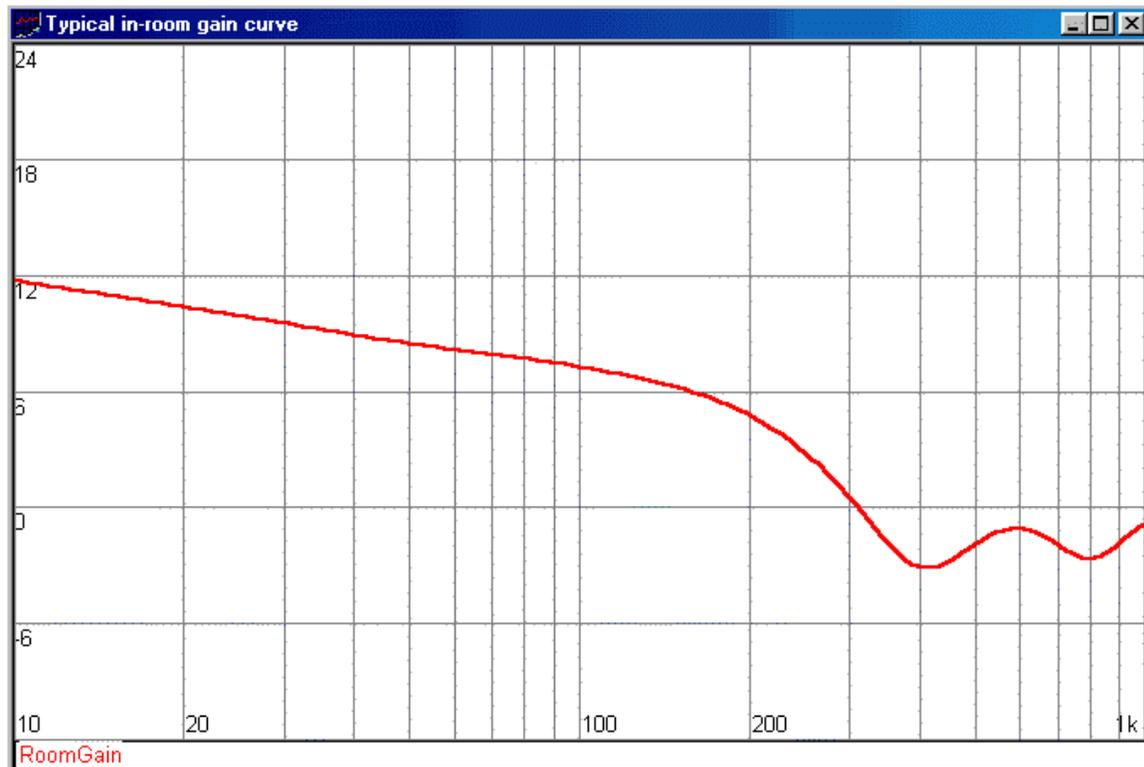
As you can see, such a room and placement within the room can provide 10 dB of gain at 20 Hz. In addition, the total gain starts well above the typical crossover point (above 300 Hz).
