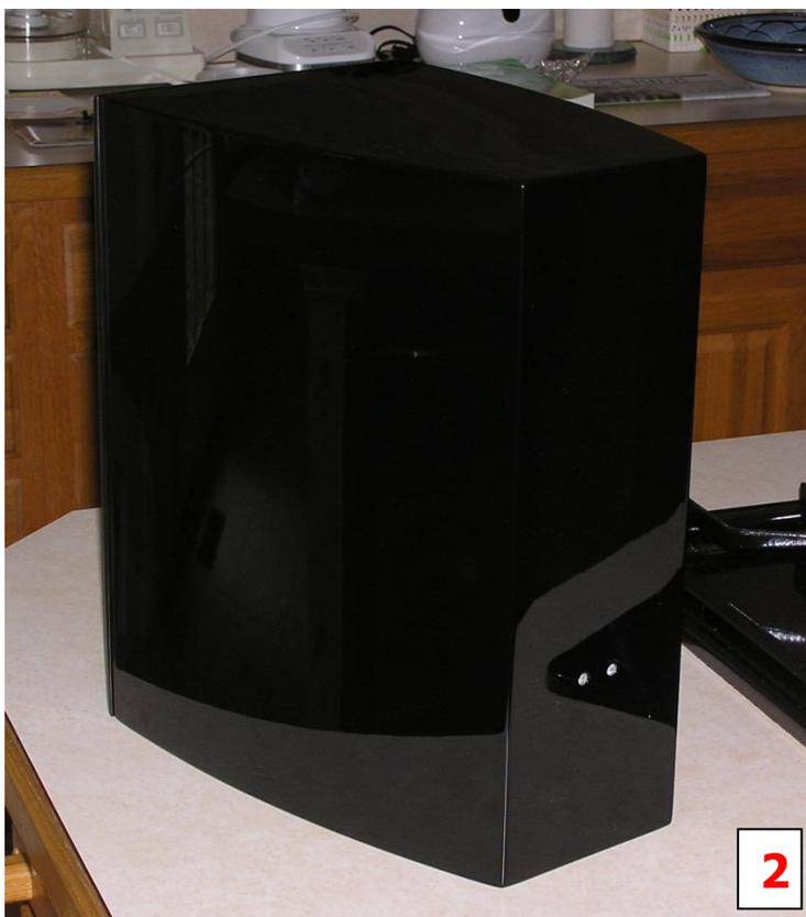
Any sturdily built cabinet with a similar internal volume ( $\pm 10\%$ ) and an 8" wide front baffle should work equally well with this design. The curved sides are not required, but they do look cool. These cabinets are not the exact same dimensions as in Dennis Murphy's drawings, but their internal volume is about the same and the front baffle width is exactly the same 8". Those are the critical cabinet dimensions.
