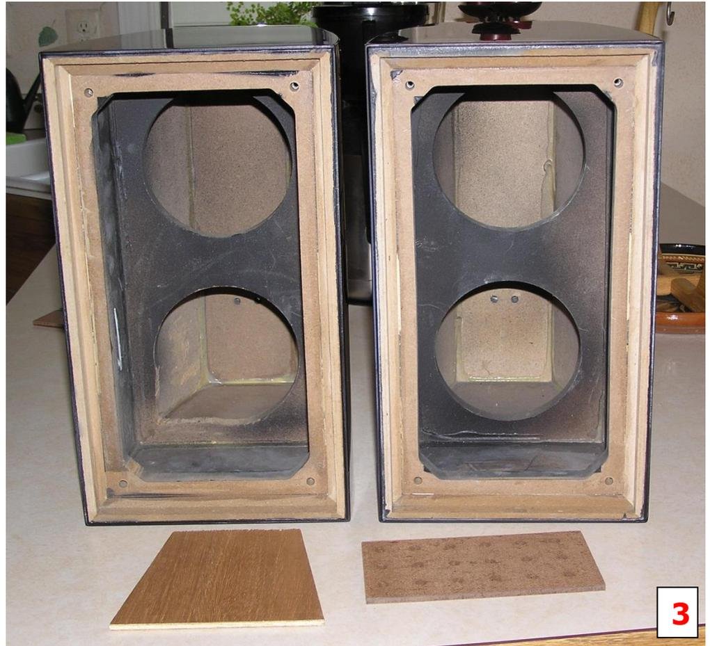
I had to cut out a notch in the lower hole of the cross brace to allow the woofer board to pass through. **Photo 3** shows one notch only on the left cabinet, but both cabinets did get modified. Later during assembly, I found that two notches were required (**Photo 15**). **Photo 4** shows the Stanley Sharptooth saw I got to do that job. The 10" blade is long enough to reach the cross brace and the teeth cut on both push and pull strokes.
