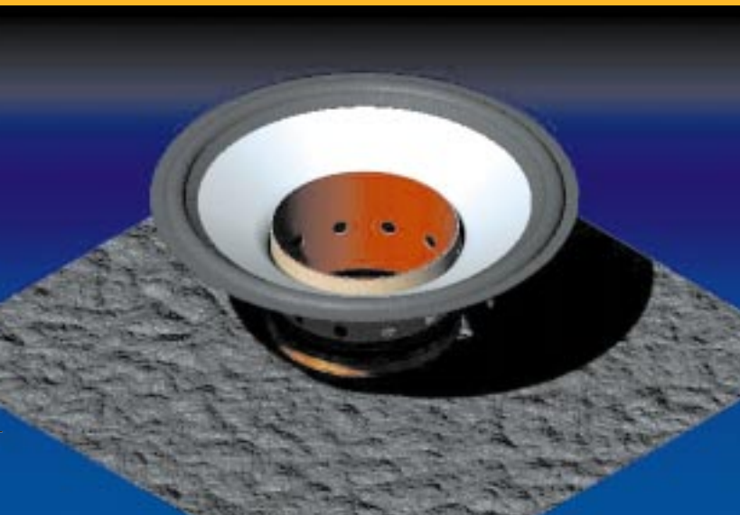
Figure 2. The computational model of the moving assembly of a loudspeaker: voice coil, voice-coil former, cone and surround. The model is used to calculate the resonant modes of the system for different cone materials.
