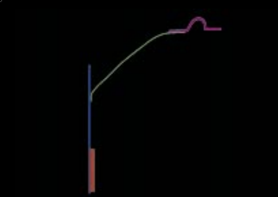
Figure 5. The shape of the first mode with a polypropylene cone, at 1500Hz.
