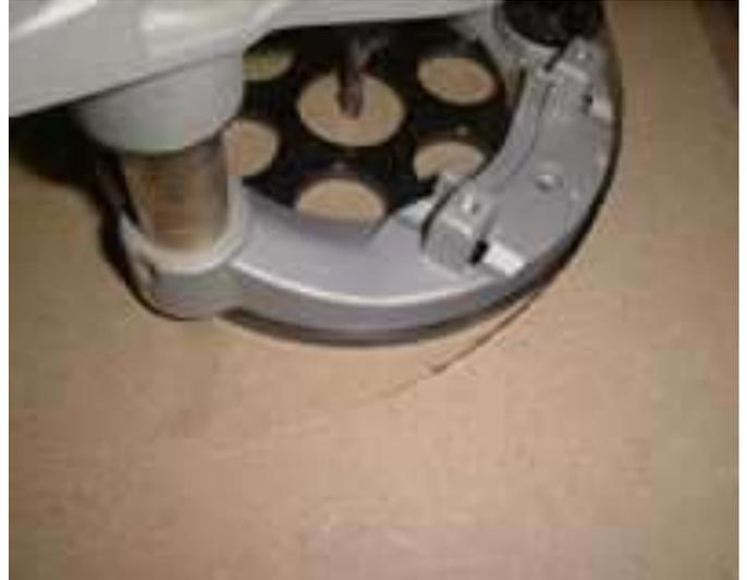
**Step 3: Use Template 2 to cut the recess on the front baffle.**
