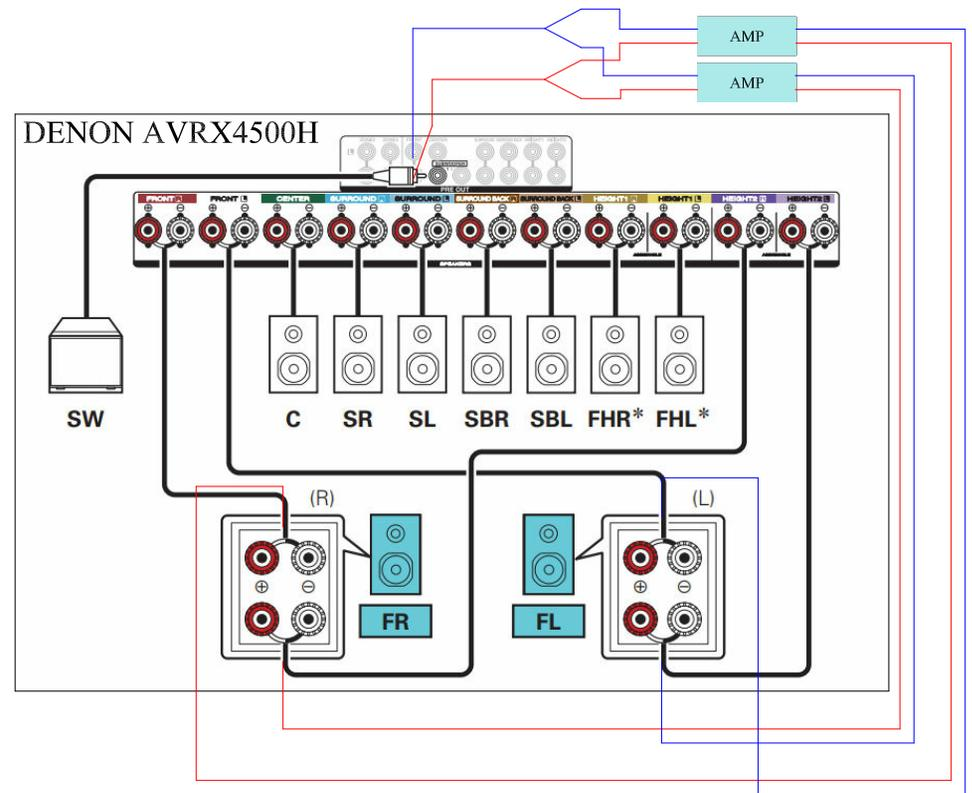
Proposed connections for using the Pre-out Front Channel with 'Y' RCA cables to feed external amplifiers
