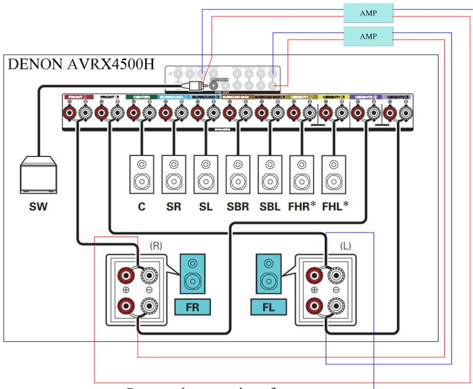
Proposed connections for bi-amp enabled AVR using external amplifiers for front channels
